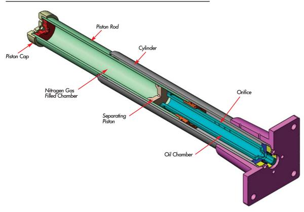
The Heavy Industry (HI) Series buffer design incorporates the proven damping system of multiple orifice patterns drilled down the shock tube length, for precise deceleration profiles, coupled with a nitrogen return system for controlled extension of the piston rod to its original position.
